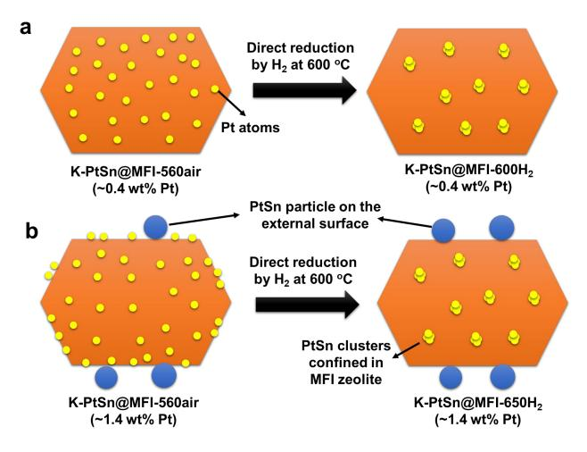
**Fig. 1.** Schematic illustration on the K-PtSn@MFI samples with different Pt loadings prepared by onepot synthesis. When increasing the Pt loading from ~0.4 wt% to ~1.4 wt%, some Pt nanoparticles will form on the external surface of MFI zeolite crystallites after reduction by H<sub>2</sub> at 600 °C.
