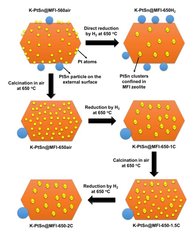
**Fig. 6.** Schematic illustration on the evolution of Pt species during high-temperature oxidation and reduction treatments. Direct reduction at 650 °C will cause the formation of many Pt nanoparticles on the external surface of MFI zeolite. After oxidation-reduction treatment, Pt nanoparticles on the external surface will migrate into the internal space and subsequently stabilized as Pt clusters in the sinusoidal channels.
