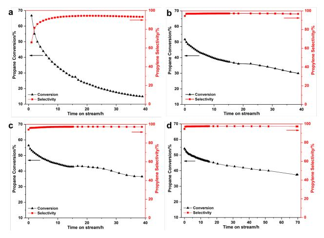
**Fig. 10.** Catalytic performance of K-PtSn@MFI samples tested under high weight-hour space velocity conditions. Reaction conditions: 20 mg solid catalyst, 5 mL/min of propane and 16 mL/min of N<sub>2</sub> as feed gas, 600 °C. All the samples were reduced by H<sub>2</sub> in the fix-bed reactor at 600 °C for 1 h before
