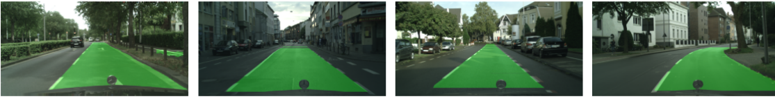
Figure 5.14: Using line detection and segmentation results for lane detection
