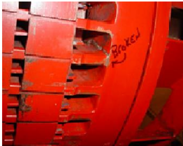
Figure 1. Illustration of: An example of industrial motor (2000 H.P) with broken rotor bars.
