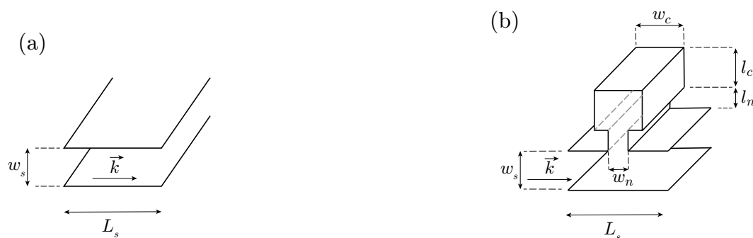
Figure 1. (a) Scheme of the wave propagation in a slit. (b) Scheme of a 2D Helmholtz resonator.
