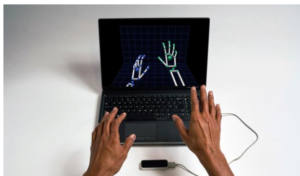
Figure 2 Leap Motion Controller recognise gesture using Skeleton Model
