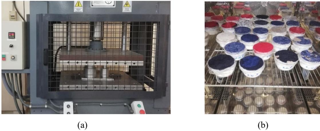
Fig. 5. Hydraulic press used for compressing molding technique (a), sample conditioned in the climatic chamber for hygric measurements (b).
