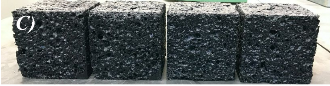
Fig. 4: Pictures of the visual appearance of the obtained materials (10 cm cubic specimens): a) Traditional cellular concrete (CA sample); b) Alkali activated cellular concrete (BA R sample); and c) One-part eco-cellular concrete (BA R -RO sample).
