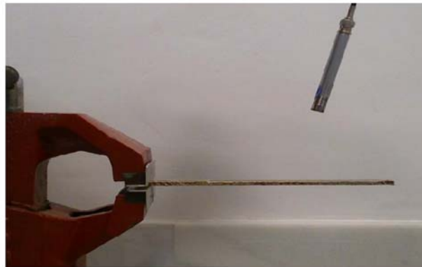
Figure 8. Experimental set-up for the vibration test.
