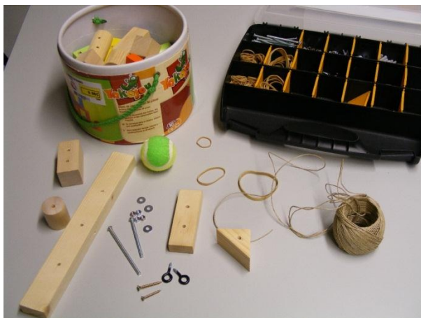
Figure 15. Wooden building blocks and joint elements for the physical-only setting.
