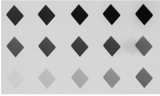
Fig. 2. HD-V2 after several irradiation times at constant beam current. Different doses generate an OD gray spectrum.
