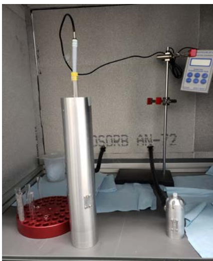
Fig. 10: Both cavities inside the Faraday cage. Vials with caps placed in cavities and temperature probe inserted through cap in large cavity
