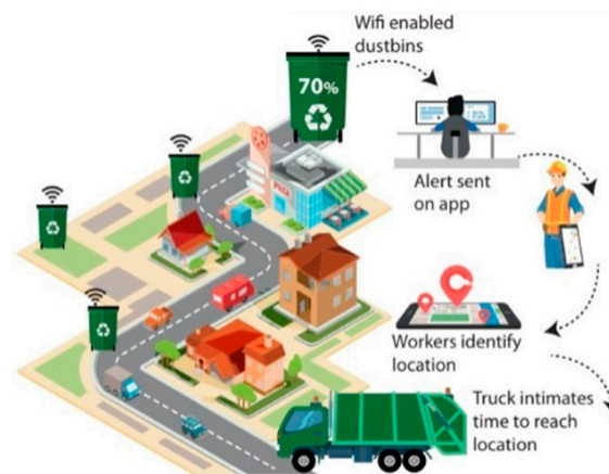
Figure 2. Overall system overview of SGCS.
