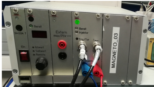
(b) Commercial injector driver (PIU injector).
