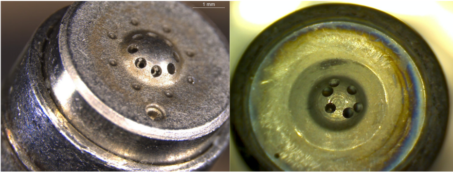
Figure 2.14: Close up picture of the injector nozzles used in this work. Spray G from ECN [26] (left), and PIU (right).
