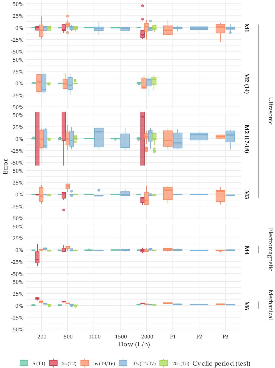
Figure 12. Error distribution under intermittent flow conditions. T2, T3, T4, T5, T6, and T7 test types. DN15. Results of T1 type tests were added as a reference.
