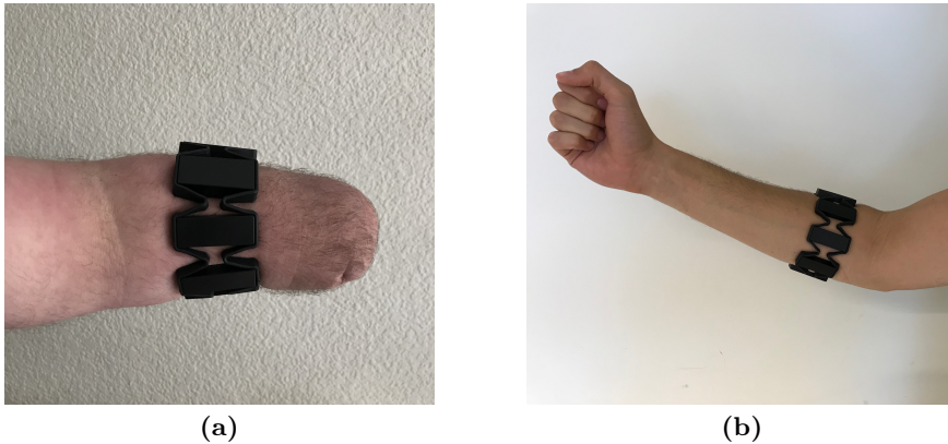
Figure 4.1: Myoelectric Armband. (a) Amputee participant using the Myo Armband. (b). Able-bodied participant using the Myo Armband.
