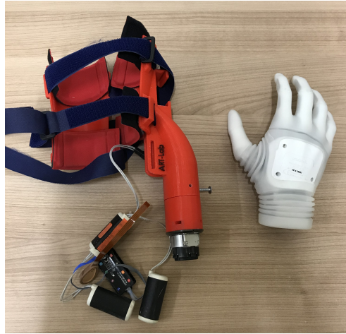
Figure 7.8: The Michelangelo Hand from Ottobock. The picture shows the prosthesis and the adapter for able bodied users manufactured by the ART-Lab.
