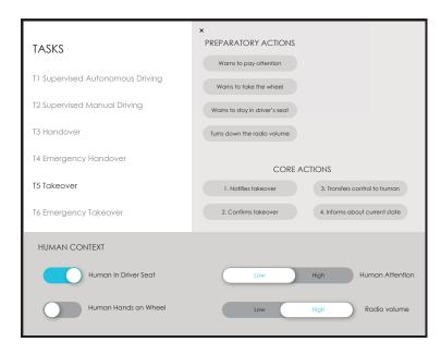
Figure 7: Web interface for the operator to simulate context and trigger the HiL actions
