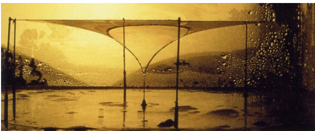
Figure 13. Soap film minimal surface with a low point made up by a loop pulled downwards. ©Atelier Frei Otto + Partner.
