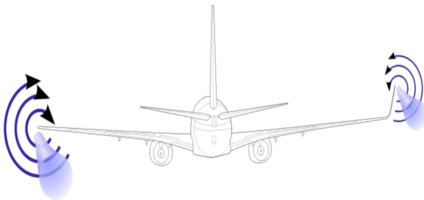
Figure 46: Reduction of vortex size with the use of winglets. [22]
