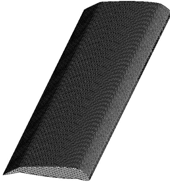
Figure 29: Wing mesh in FlightStream.
