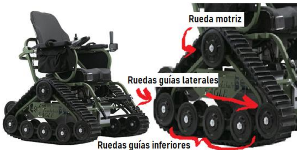
[Imagen 25]. Sistema oruga con forma triangular - http://actiontrackchair.com/trackchair-eagle/ - 2021
