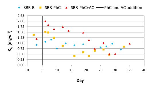
Figure 5. Evolution of sludge production of SBRs. Vertical line indicates the day in which PhCs and AC were added.
