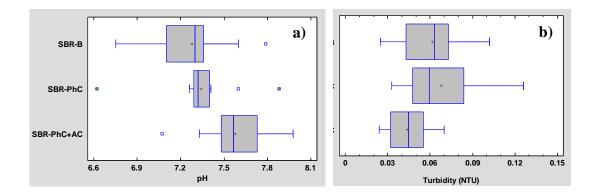
Figure 3. Tukey diagram for pH (figure a) and turbidity (figure b).
