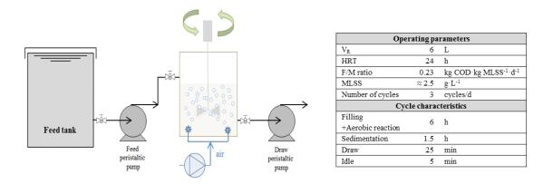
Figure 1. SBRs characteristics and configuration.
