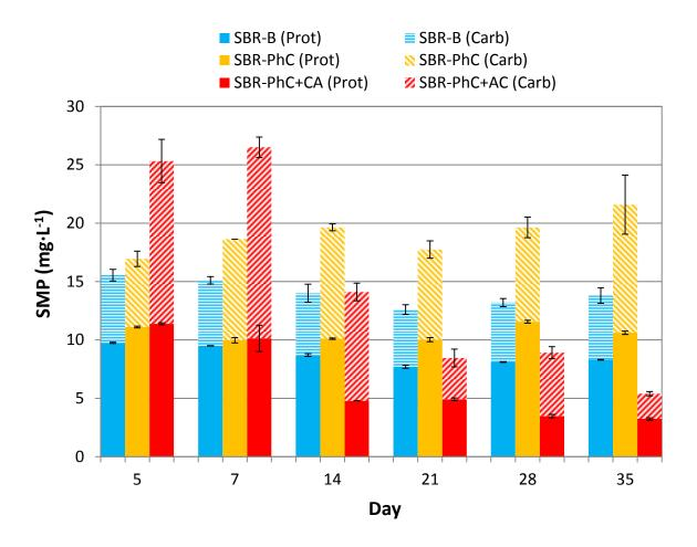
Figure 6. SMP concentration in SBR-PhC and SBR-PhC+AC. SMP are plotted as the sum of proteins (Prot) and carbohydrates (Carb) concentrations in each reactor.
