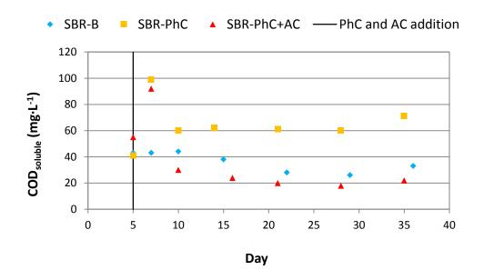
Figure 4. Effluent COD evolution of SBRs. Vertical line indicates the day in which PhC and AC were added.
