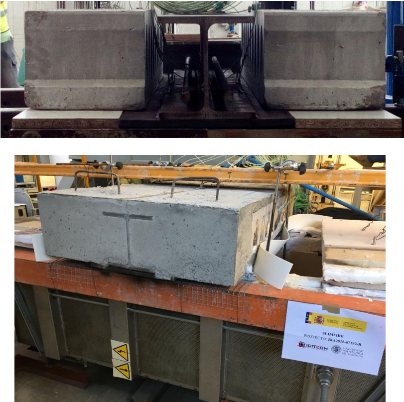
Fig. 16. Experimental setup for elevated temperature slim-floor tests at the Polytechnic University of Valencia (Spain).
