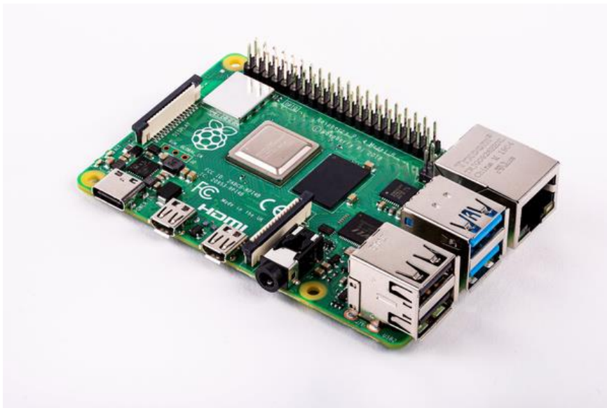
Figure 6: Raspberry Pi 4 Model B 1 . General view of the single computer board
