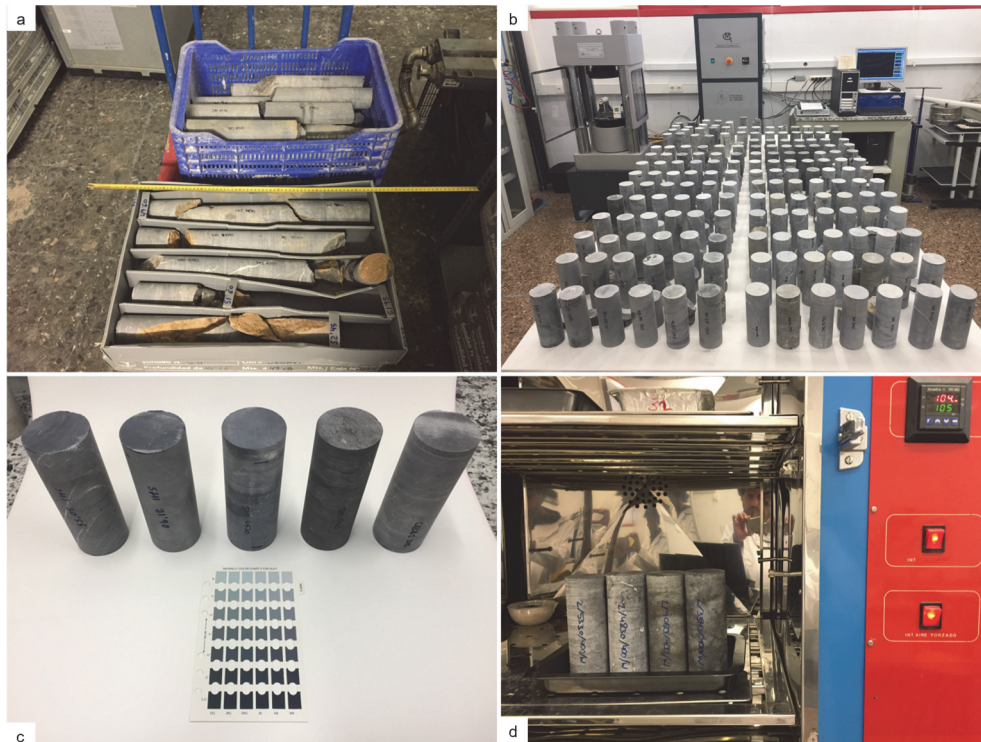
Figure 1.2. Core samples taken from horizontal survey boreholes (a) and cut samples with a slenderness of 2.5 (b). Slight changes in the grey tone and very thin veins of calcite observed in the tested samples (c). Heating of the samples at 105°C for the determination of the intact rock properties (d).
