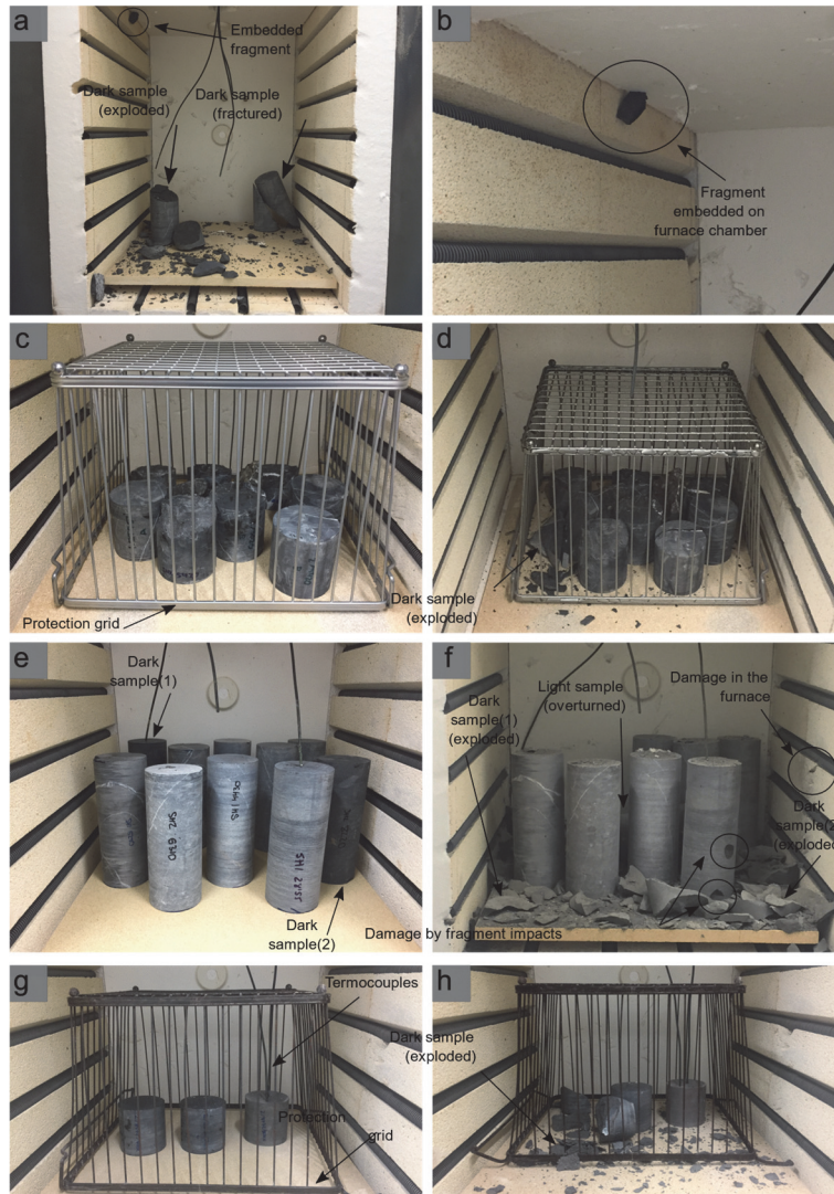
Figure 3.6. (a) Dark samples exploded or fractured when heated at 400 °C. (b) Detail of the fragment embedded in the furnace chamber due to the violence of the event shown in (a). Dark samples before (c) and after (d) heating at 400 °C. Note the protection grid used to preserve the furnace. Dark and light grey cores before (e) and after (f) heating at 500 °C. Note that only dark cores exploded, and their fragments overturned and damaged the surrounding light grey samples and the furnace chamber. A new set of dark samples before (g) and after (h) heating at 500 °C using the protection grid. The temperatures were being registered using thermocouples when one sample exploded.
