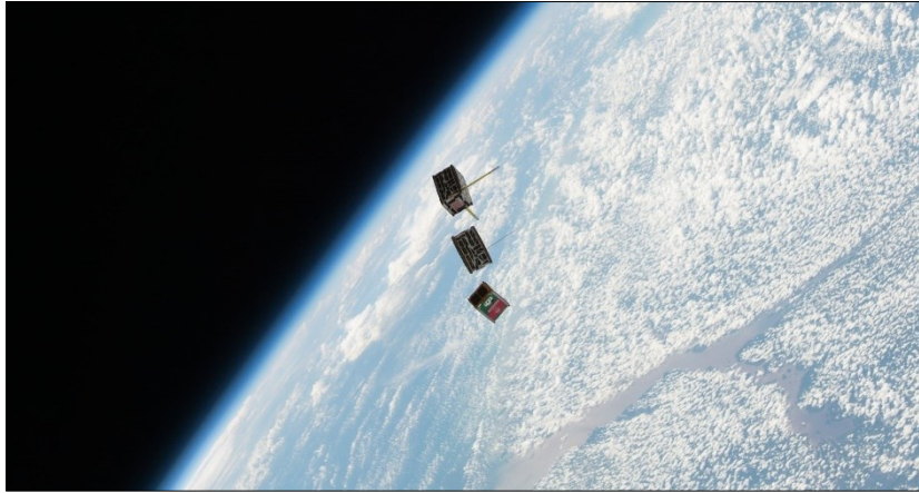
Figure 1.1 CubeSats fly free after deploying from International Space Station 1
