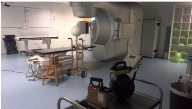
184 Fig. 10. Experimental measurements with neutron detectors.
