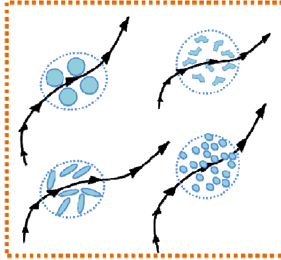
Figure 2-11: A schematic showing treatment of particles using the Lagrangian approach (Adapted from Vujanovic et al., 2009 [43]). Each dotted circle represents for a parcel.
