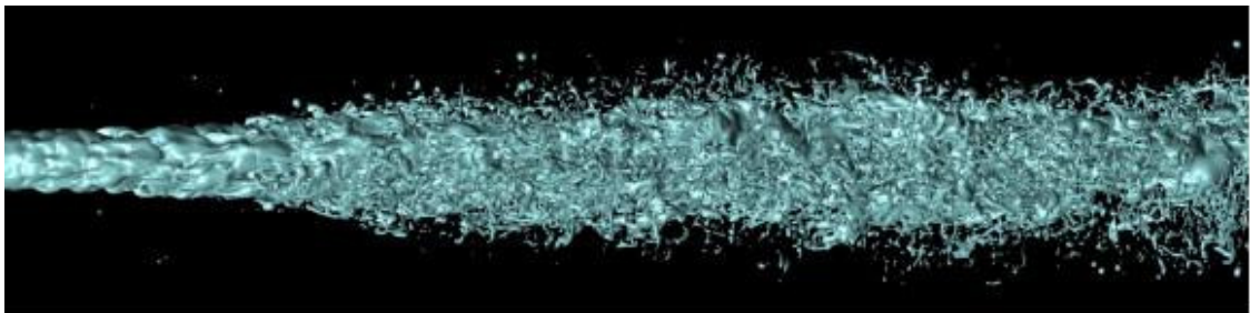
Figure 2-9: DNS simulation of Diesel sprays. Computational domain is 0.3 mm x 0.3 mm x 2.2 mm, grid size is 128 x 128 x 896, D_0 = 100 \mu\text{m} , U = 100 \text{ m/s} , \rho_{inj} = 696 \text{ kgm}^{-3} , \rho_{cha} = 50 \text{ kgm}^{-3} , computing time 10,000 h on 14 processors (Lebas et al., 2009 [42]).
