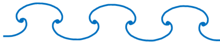
Figure A-8: Schematic Pattern of the Rayleigh-Taylor instability (Dhainaut, 2002 [13]).
