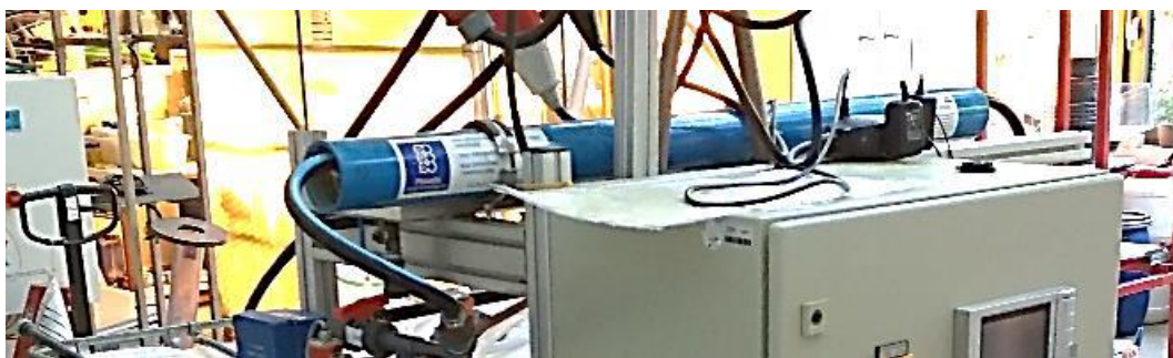
Figure 3.3. Close-up view to the cylindrical vessel which contains the membrane
