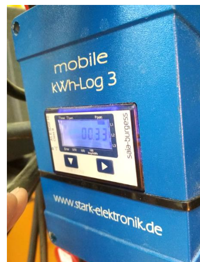
Figure 0-6 - Energy meter and control sequence to read power consumption
