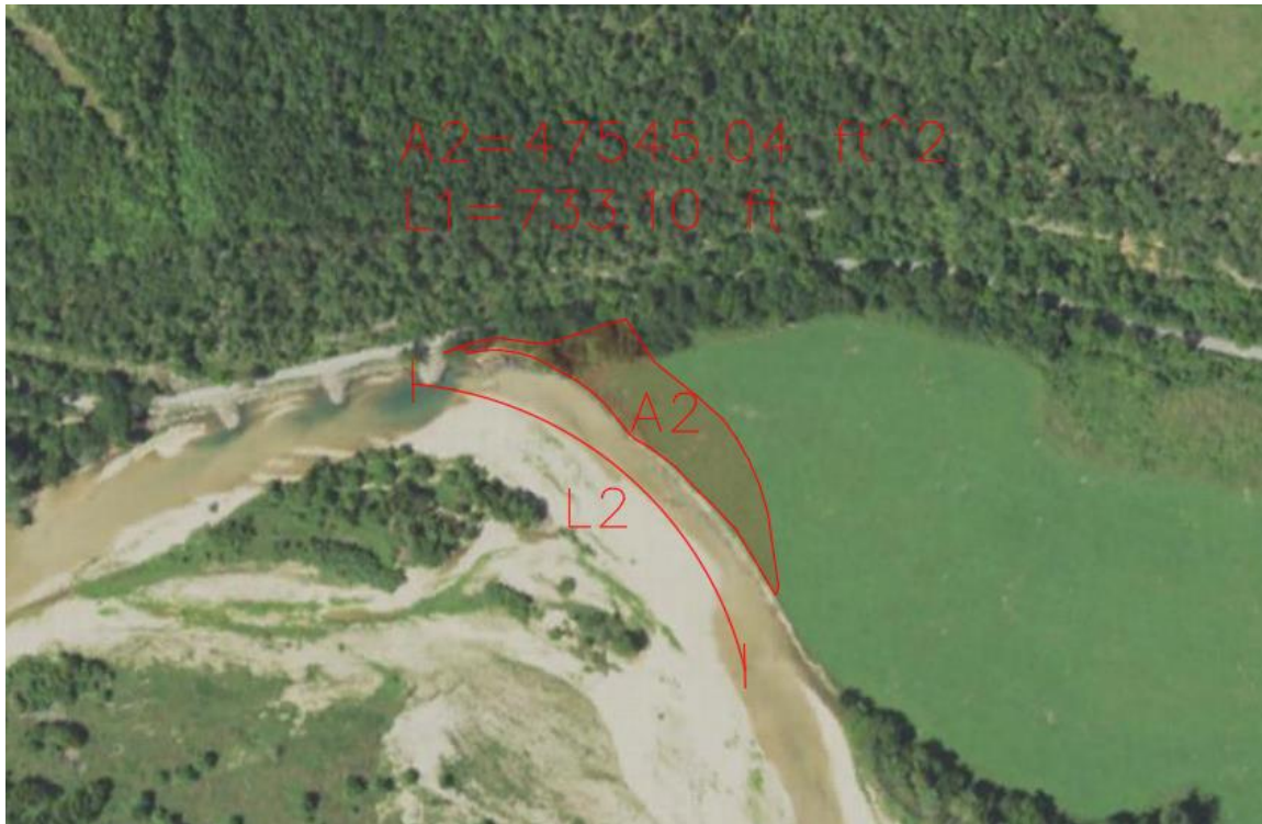
Figure 28 (appendix)– Reach 2, 2019 aerial imagery, showing the erosion in the following 2 years
