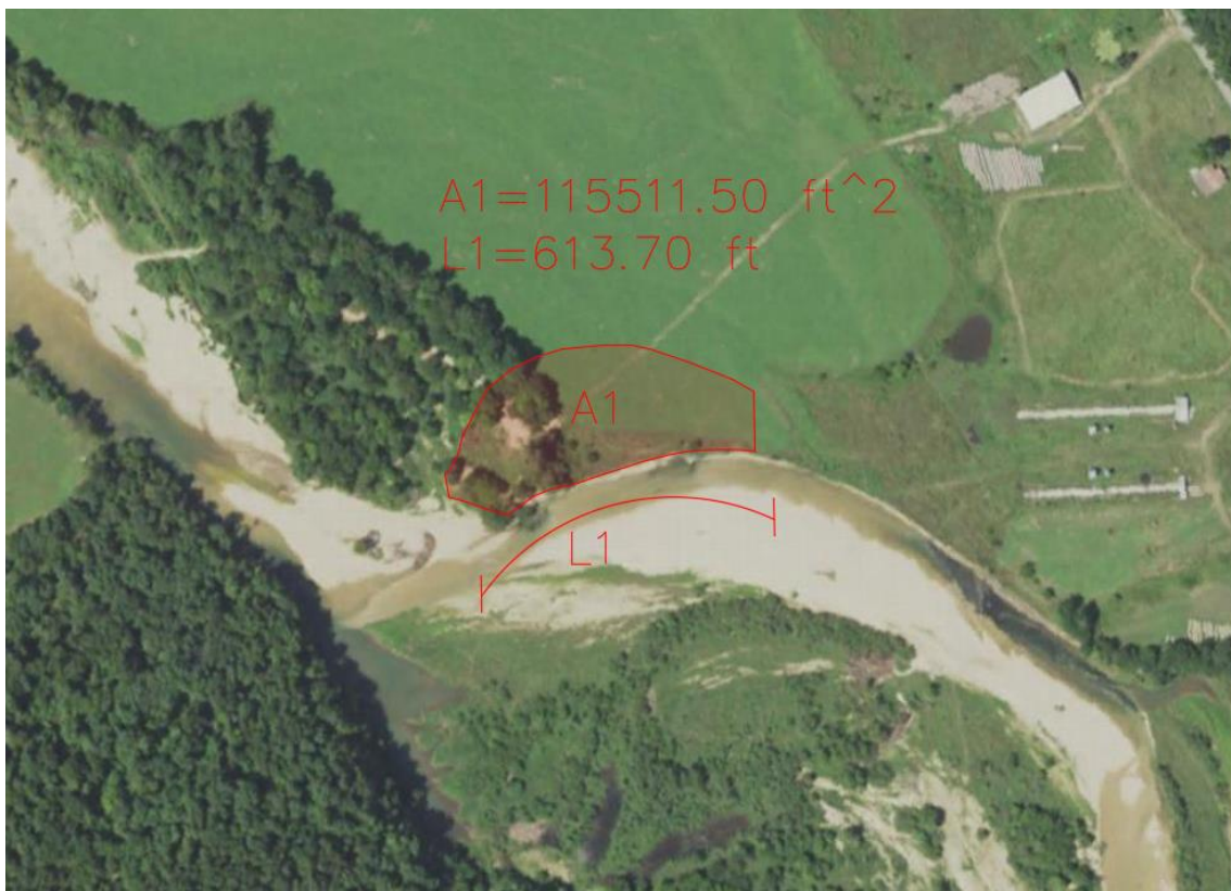
Figure 26 (appendix) – Reach 1, 2019 aerial imagery, showing the erosion in the following 2 years
