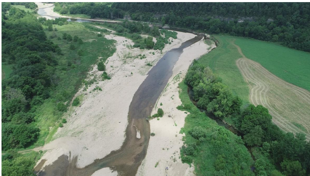
Figure 50 - Reach 2 (at the far top right side), 2021 drone picture showing how the river is trying to increase its length by meandering more but the road is in the way.
