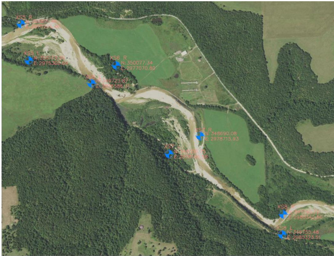
Figure 24 – GPS Coordinates of the 2021 survey used for the cross-sections (Oklahoma North State Coordinates)
