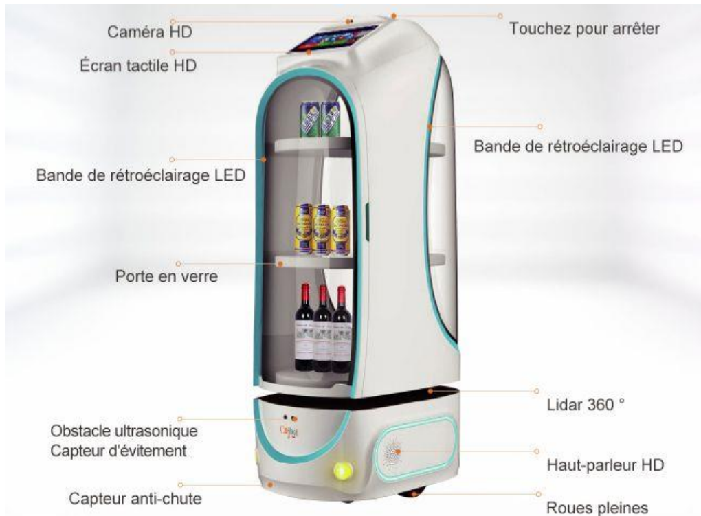
Figure 51: CSJBot vender robot specifications
