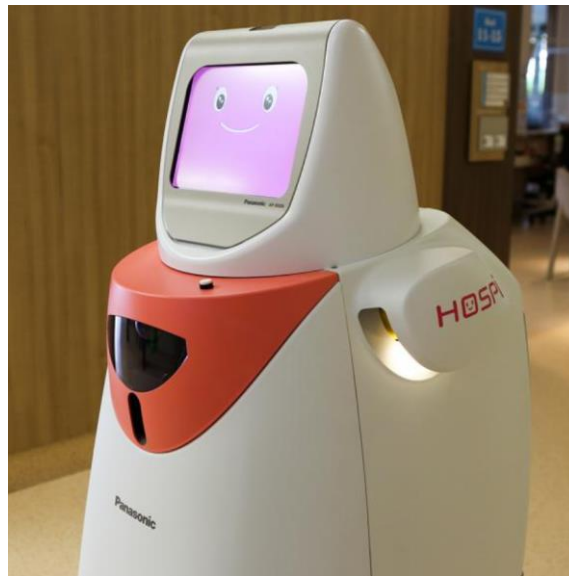
Figure 22: HOSPI – Hospital delivery robot
