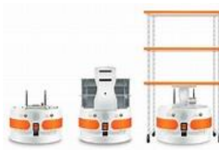
Figure 44: Load variants in PAL delivery robot
