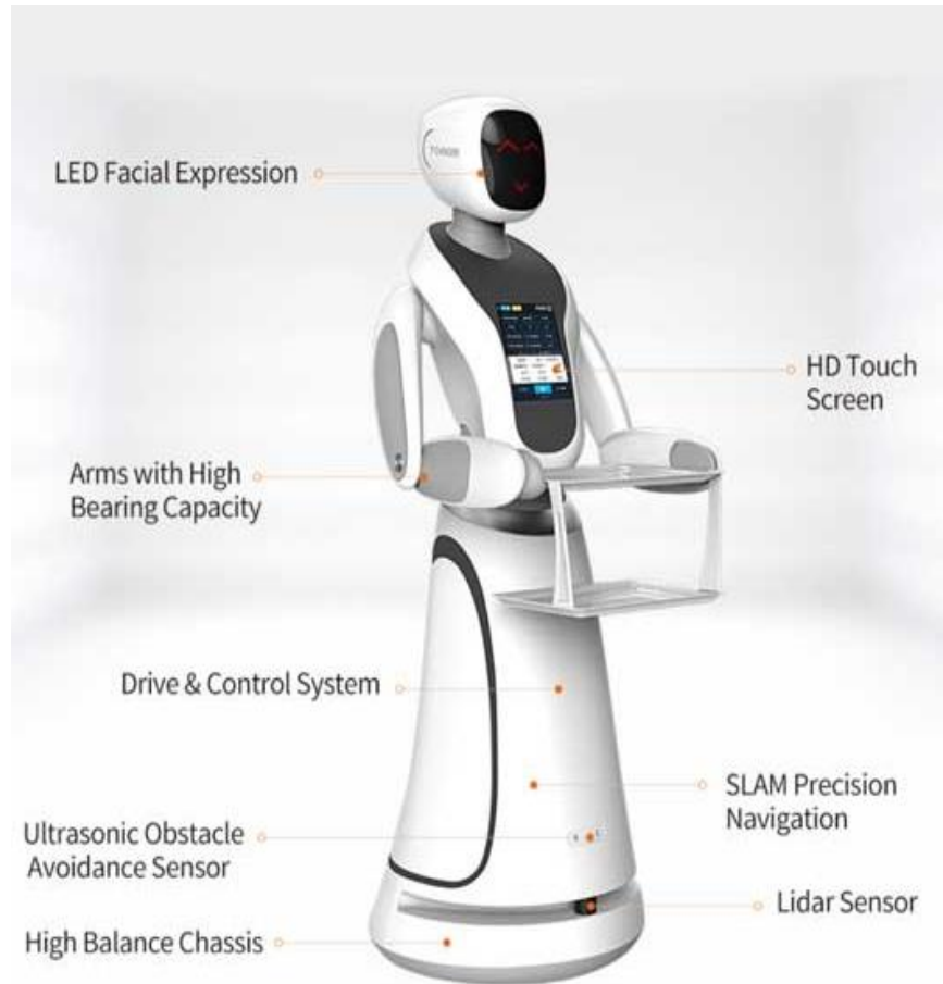
Figure 47: Amy waitress robot specifications
