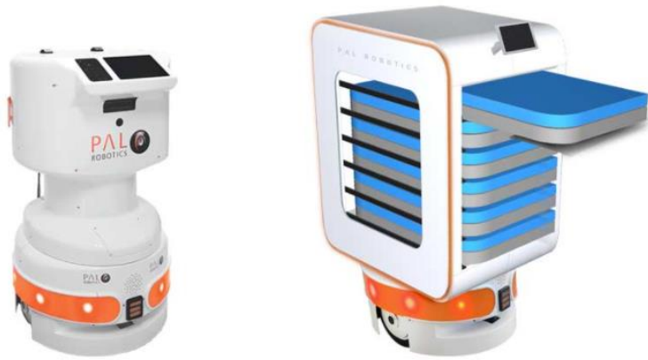
Figure 43: PAL Robotics delivery robot
