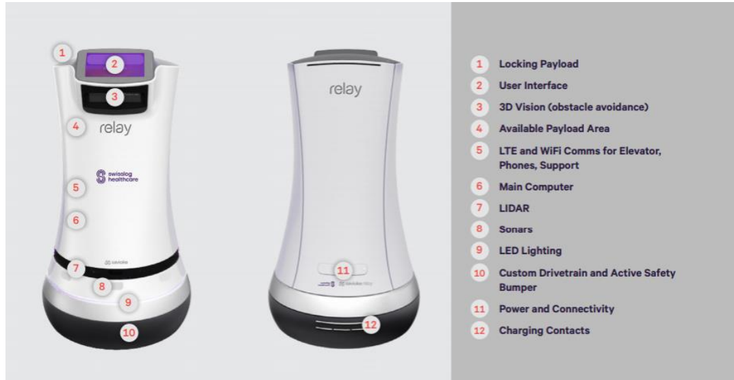
Figure 15: Specifications Savioke Relay Robot
