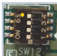
Figure 5.2: Switch 12 configuration for UART debug link
