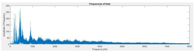
Fig. 26 FFT results of data from microphone 2
