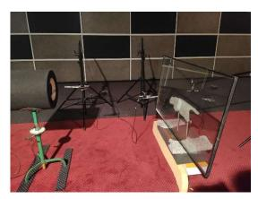
*Fig. 14 Photo of the measurement setup from the session with a glass window*
