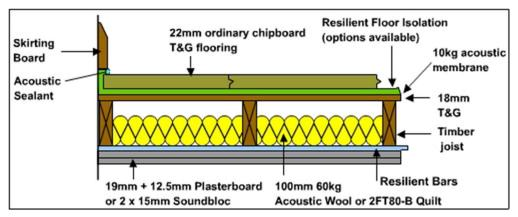
Fig. 21 Diagram of a floating floor (Noise Control Soundproofing and Acoustics, n.d.)
