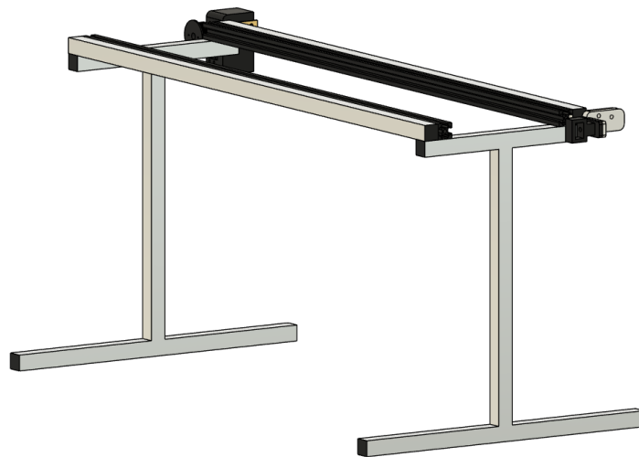
Figure 21. Belt transmission mechanism attached to frame
