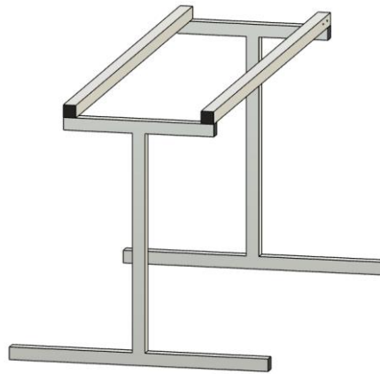
Figure 12. "I"-shaped robot-lifting aluminum structure
