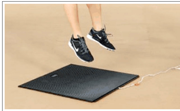
Figure 2.8: Just Jump vertical jump measurement method
