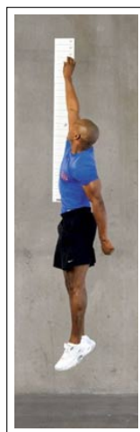
Figure 2.5: Wall mounted vertical jump measurement method
