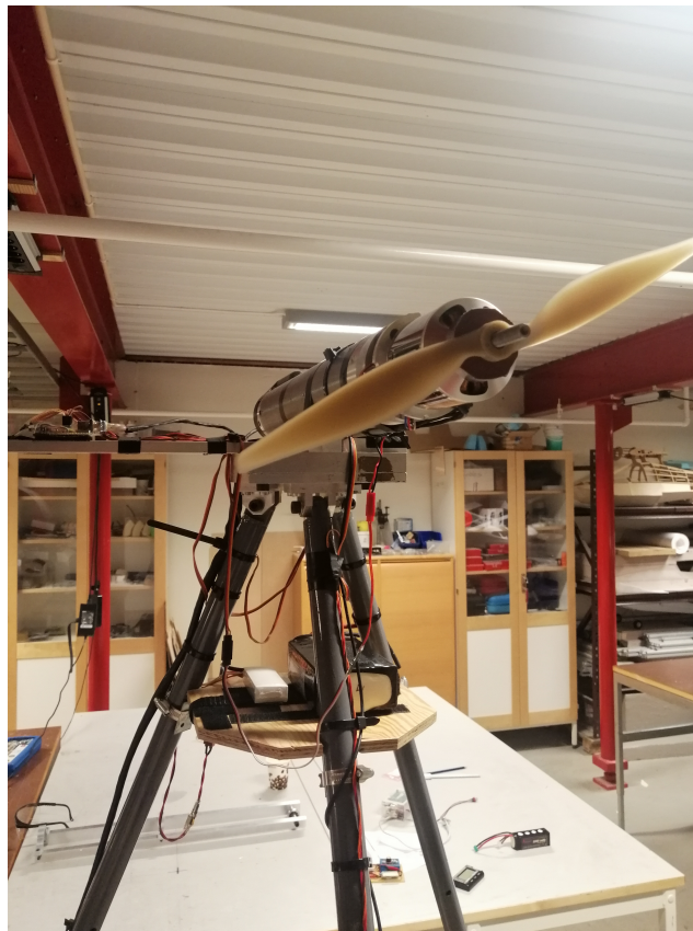
Figure 13: Motor and propeller mounted on the testing rig
