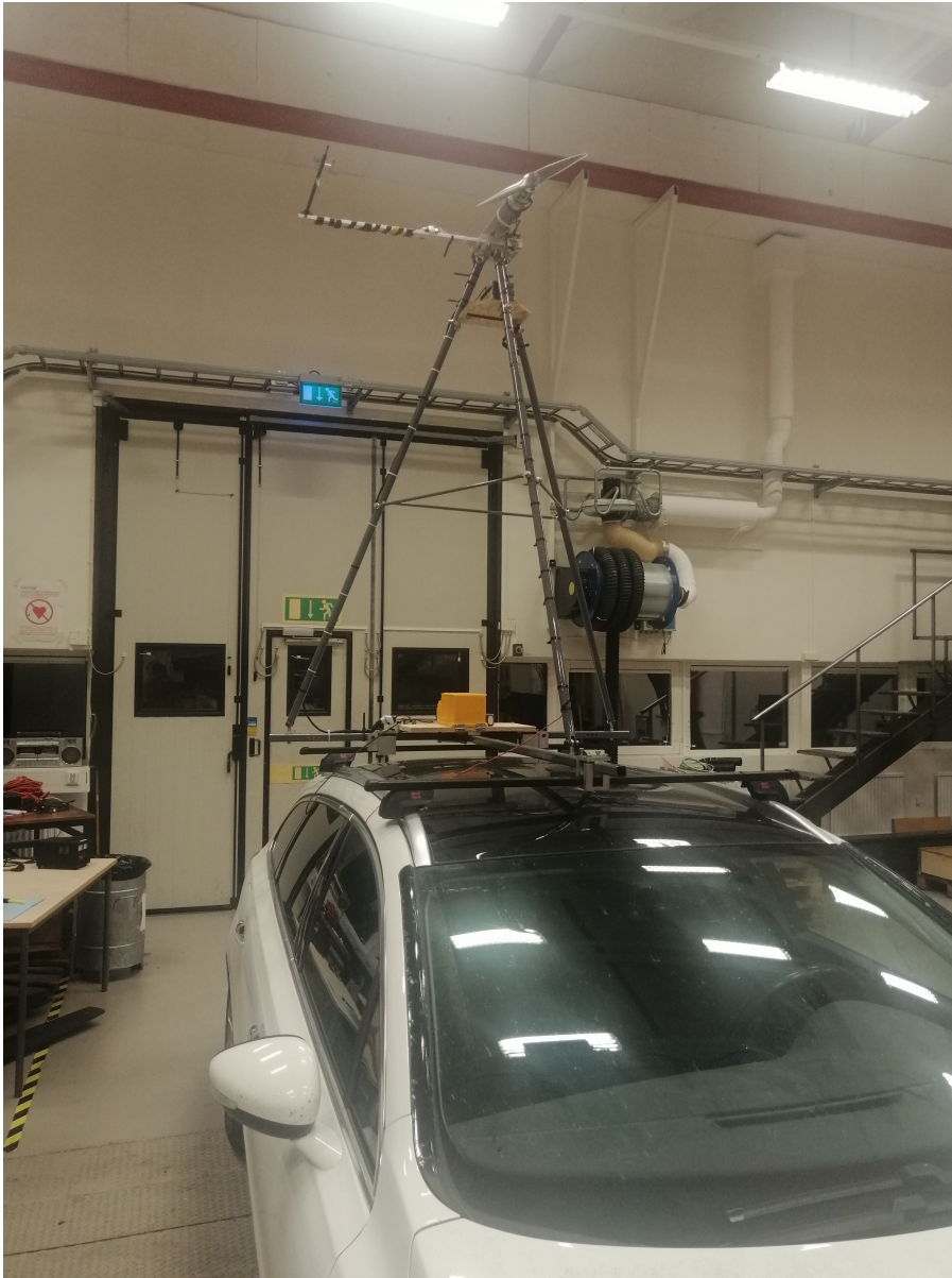
Figure 15: Testing rig mounted on car roof
