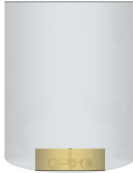
Figure 3.4: Model used with the interface separating the two designated regions. Spinning section marked in yellow.
