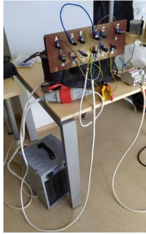
Figure 18: Heater (H) = Transformer 380/113 V + heater with fan
