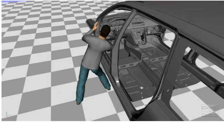
Figure 13. Example of a simulation with IPS IMMA (Image obtained from https://industrialpathsolutions.se/ ).
