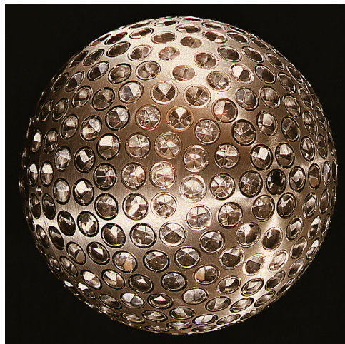
Figure 4: LAGEOS-1 satellite with corner-cube reflectors [1]
