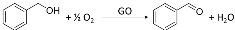
Fig. 20 Aerobic oxidation of benzyl alcohol to benzaldehyde using GO as metal-free catalyst.
