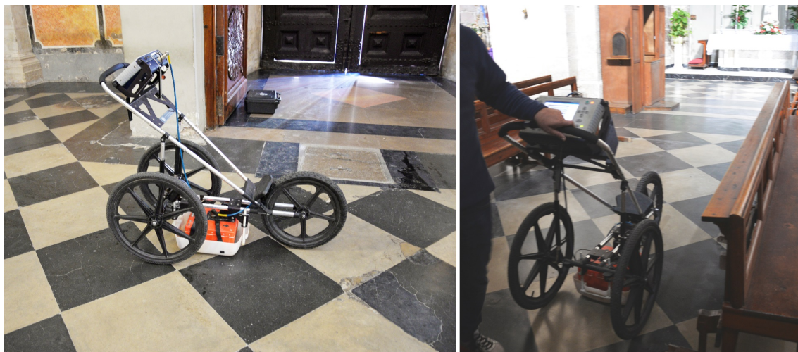
Figure 3. GPR Sir model 3000 with 200 MHz antenna used in the church of the Asunción of Lliria.
