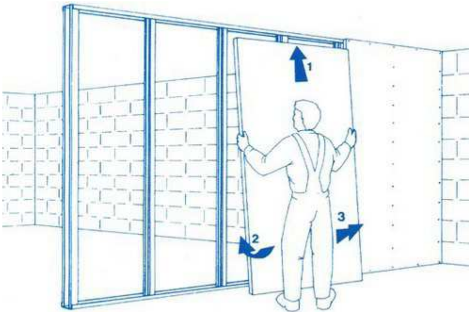
Figure 21. Placement of plasterboard
