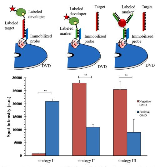
**Fig. 3.** Comparison of labelling strategies for DVD biosensing. I: simple hybridisation of the labelled amplification products (digoxigenin); II: indirect competitive hybridisation of the amplification products and labelled marker (digoxigenin); III: direct competitive hybridisation of the amplification products and nanogold-labelled marker. \*\*: p-value < 0.01.
