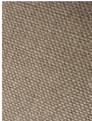
Figure 1. Basket weave (2 × 1) flax (BF) used for manufacture biocomposite specimens through compression molding.
