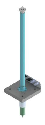
Figure 3.7: Variation G1: Shaft inside the tower
