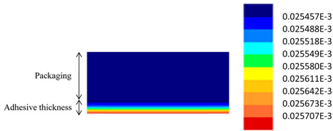
Fig. 11. Cross section of the sensor showing the strains in the X-direction. Adhesive thickness is 100 \mu\text{m} , adhesive Poisson's ratio is 0.4.
