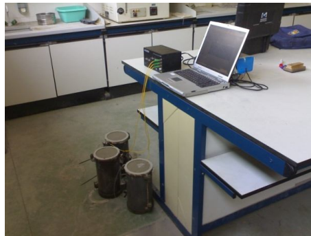
Figure 3: Interrogator sm125-500 , computer and instrumented specimens with Optical temperature sensors and termocouples.
