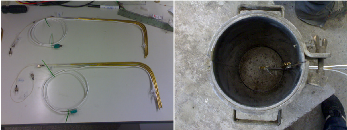
Fig. 3: Two sets of sensors fabricated, on the left. Location of these sets inside the cylindrical mould before concrete pouring, on the right.
