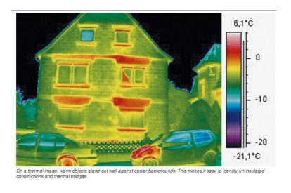
Thermal image example. For the preliminar report we need to take pictures of each critical area in this case for the following connection: floor slab/external wall.
