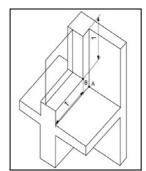
Illustration of the distances of the cut-off planes from the thermal bridge in point B (EN ISO 10211).
