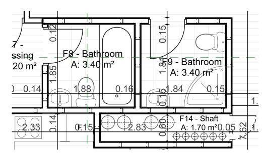
Penthouse - Arrangements of pipes in the shaft
