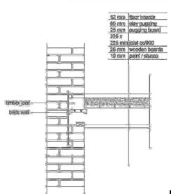
Floor slab/External wall connection
