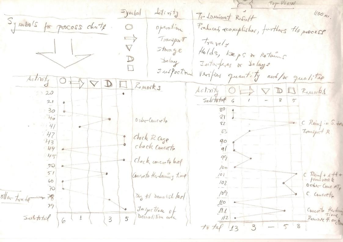
Focess & and Process Chats Brimetral pile foundation Dis til find old foundation
