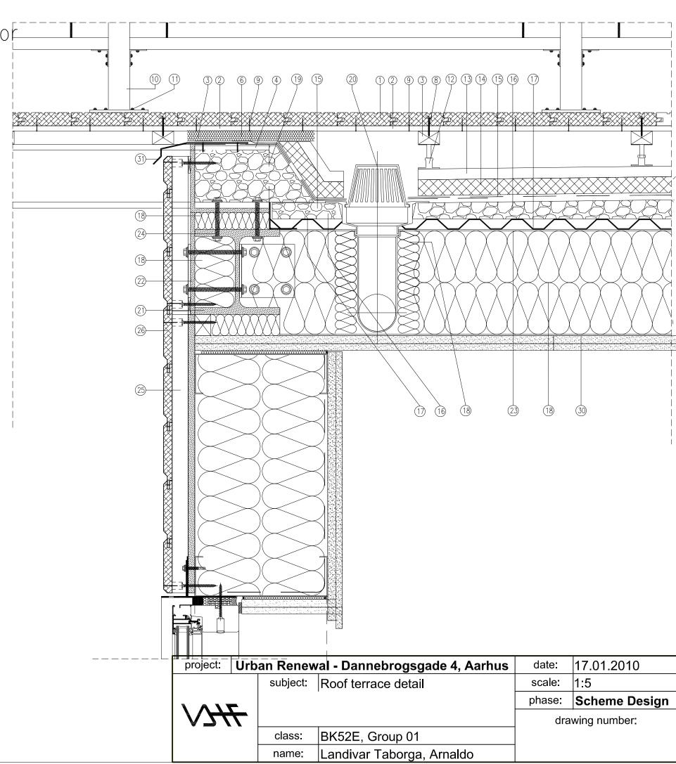
Roof terrace floor-connection with kitchen floor (vertical section) Sc 1:5
