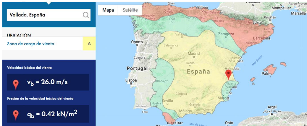
Figure 54. Wind speed and dynamic pressure according to the location of the installation. Source: Dlubal (based on DB SE AE)
