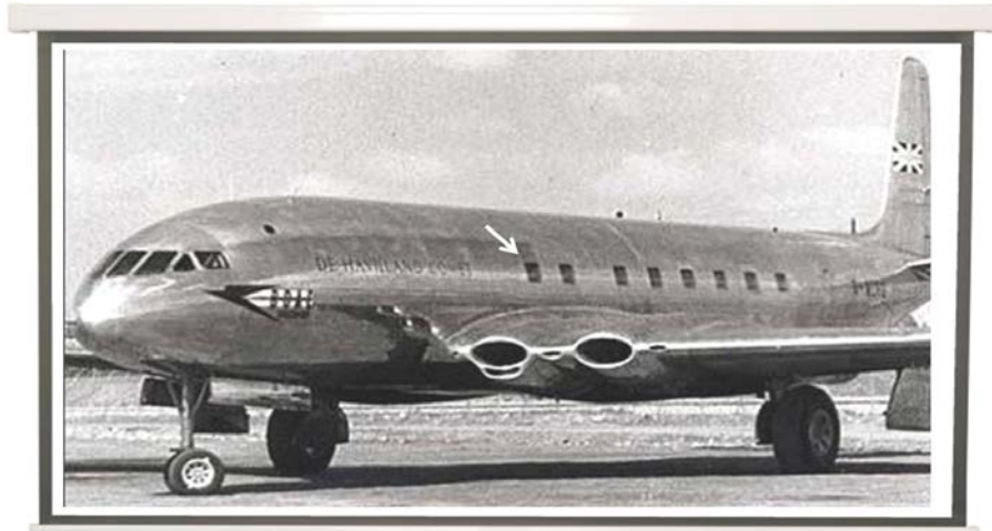
Figure 7. First version of the Comet plane that used riveted windows with square shapes of sharp vertices.
