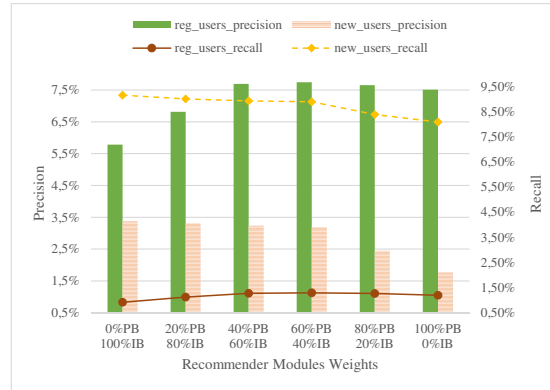
Fig. 3: Precision and recall comparison of regular users and new users, using different LRS modules weights.
