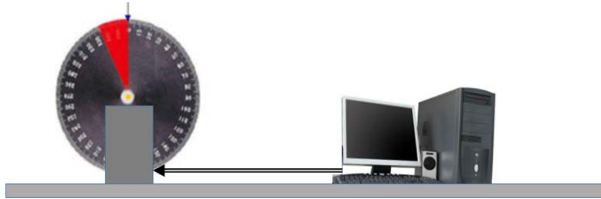
Figure 2. Computer-based control of the angular position of a servomechanism where rotational position is measured by an encoder.
